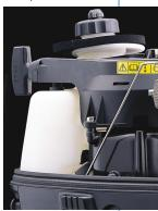
The pilot water hole is located upstream of the cylinder to confirm that there is water circulating soon after the motor is started. The pilot water inspection tube is removable to permit cleaning of the tube and the attachment of an optional connector allows freshwater flushing of the cooling system.
